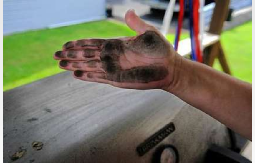
Residual DPM after ventilation dilution and vehicle treatment
